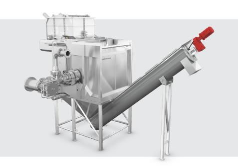
Discover Kiremko Quality The STRATA Invicta® sets the new standard in steam peeling systems, offering the highest yield at the shortest possible cycle times. It peels potatoes thinner than any machine, removing only the skin with a minimum of cooking ring!
