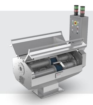
Discover Kiremko Quality The Kiremko QuadraFlow hydro cutting system transports your product in water to the knife block. Due to the ingenious transport system, the potato passes through the grid of razor-sharp knives at high velocity. Damage to the product is minimal whilst maintaining the dimensional stability and cut quality. Over many years Kiremko has optimized this technology. The stability of your process and the quality of your product are our goal.
