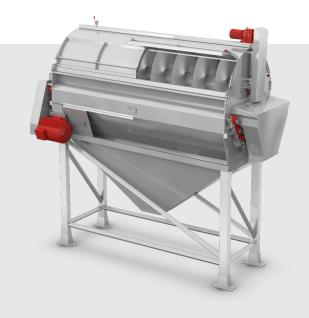
The Kiremko brush machine removes peel from the potato. A platform of four, six or eight rotating brushes effectively removes and separates the peel without causing any damage to the product. The brush machine fits seamlessly with the Kiremko steam peeler. This machine runs in many production lines worldwide.
