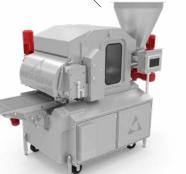
The Nex-Gem+ forming machine is an ultra-modern rotary former, which has been provided with numerous exceptional extras such as the 'Quick Change Inserts', a very swift way to exchange forming tools without the need of any special tools.
