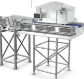
The PeelGuard® is an optical measuring and weighing device to detect residual peels and green or black spots and control your steam peeler.
